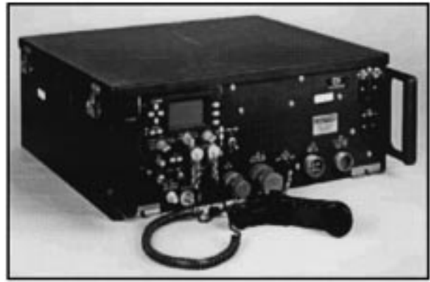
Fig. 2. AN/VRC-100 ground/vehicular HF transceiver (courtesy of Rockwell Collins).
